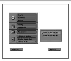
**96KHz**  $\Rightarrow$  **48KHz:** Even in case of 96 kHz digital signal, the DVD Changer will deliver 48 kHz signal out.
